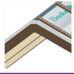
6.2 On the other side of the roof, roll out the BreatherQuilt and butt-joint to the first piece.
