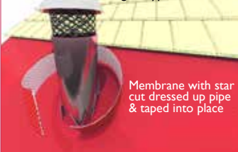
Fig. 14 Typical vent detail
