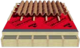
Fig.10 Warm Tiled Roof Detail
