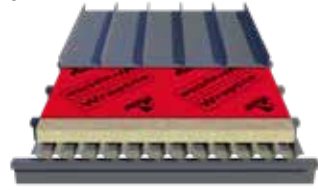
Fig.11 Warm Metal Roof Detail
