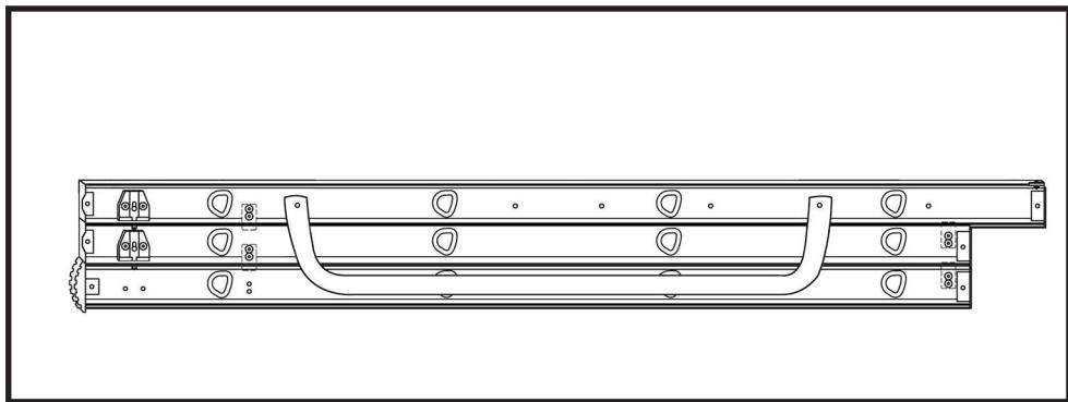
**UK** The handrail (A1) can be fitted to either side of the rear frame of the ladder.
