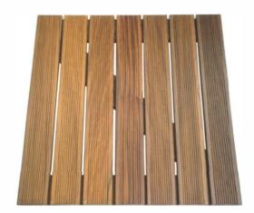
Pre-assembled 500x500 mm, 30 mm thick deck tiles in lpe wood, each made up of seven 15x67x500 mm boards, to create an anti-slip flooring surface, and three 15x67x500 mm battens for the substructure, positioned in a "Z" formation.
