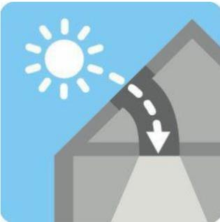
The **flexible** tunnel is ideal for distances between roof and ceiling from 0.4 to 1.5 m.
