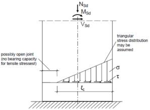
Figure 3.Determination of the compressed part of the wall
