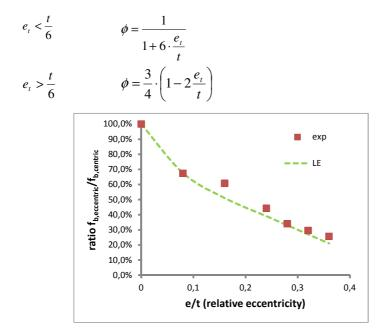
Figure 2 Capacity reduction factor for masonry with Perinsul HL thermal break unit
