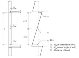
Figure 1 Bending moments in vertically loaded masonry wall
