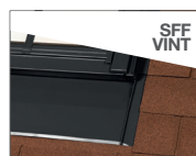
FLUSH FLASHING FOR SLATE For 40 mm recessed installation into slates and flat roofing, up to 8 mm (max overall thickness is 16 mm)
