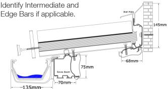
Lay taped poly sheets into Bars. Gently tap Wallplate Top Caps down onto poly sheets. Gently tap Bar Top Cap down onto sections to correct positions. Glazing deduction for
