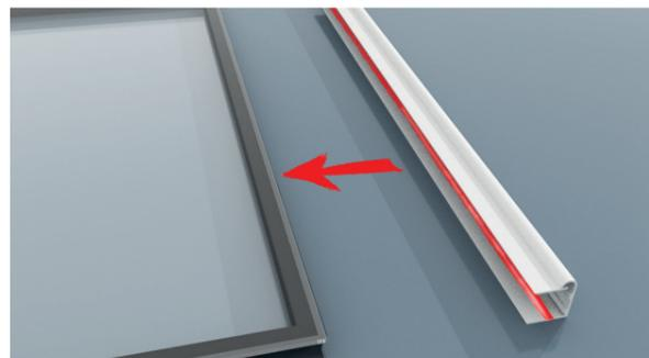
**15** Apply a bead of sealant to glazing end closer and fit centrally to glass units.
