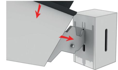
**8** Lift the hip rafter and offer the bracket up to the slot in the box ridge at an angle. Insert the bracket and rotate rafter down into position.
