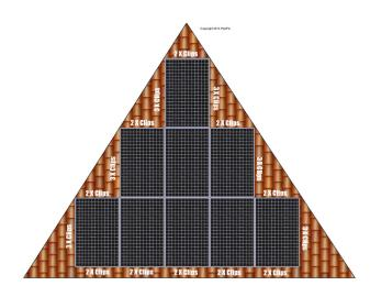
SolarFix Clips Typical 9 panel layout. Demonstrates number of clips required. Long edge = 3 clips Short edge = 2 clips Total Requirement = 36 clips Use 1 clip per 450mm of panel Edge (approx.)
