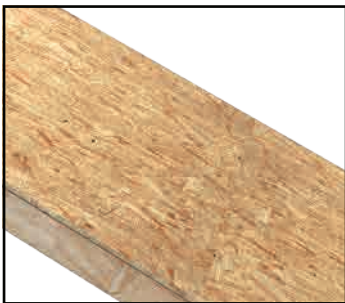
Roof deck (OSB)
