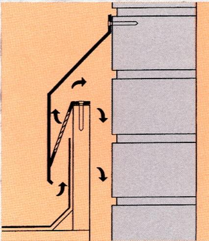
*RAV-FL in position showing ventilation path over the felted timber kerb upstand. Battens fixed vertically at one metre centres ensure the requisite ventilation aperture between upstand and masonry.*
