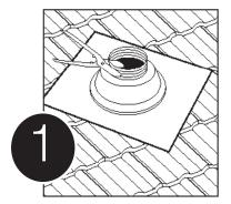
Trim the rubber boot to suit pipe size. Ensure surface is clean and dry before application.
