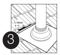
For tile roofs, remove the top backing strip and fold 5-10mm of the top of the flashing up over itself creating a dam and affix under the upstream tile.
