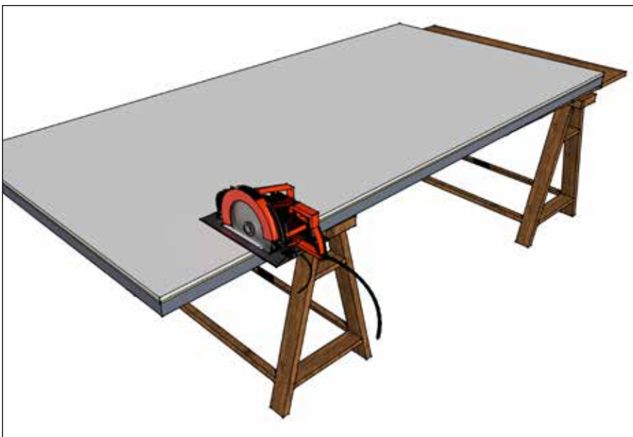
Fig. 2 Cutting Spacetherm WL boards
