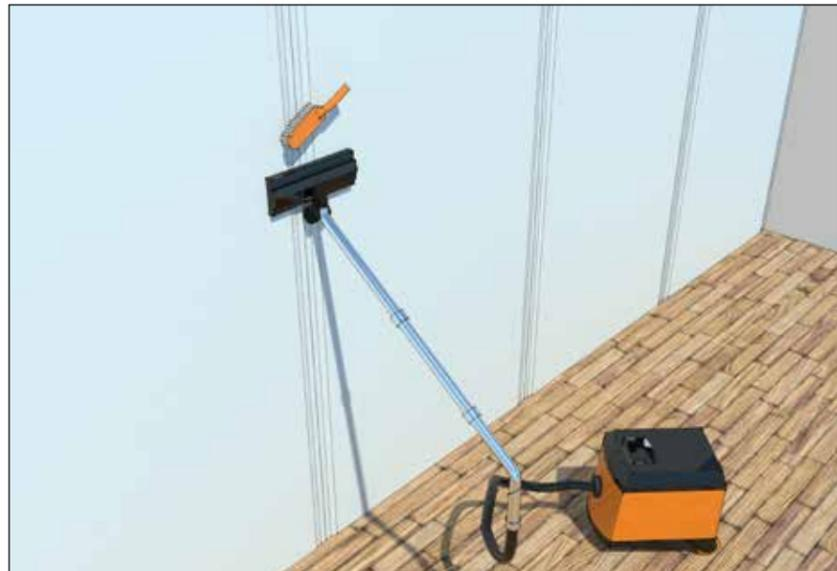
Fig. 7 Preparing Spacetherm Multi Surface for jointing
