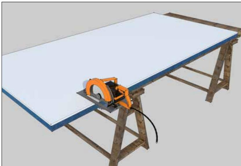
Fig. 2 Cutting Spacetherm Multi boards
