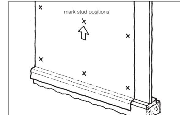
3 Ensure lowest structure of wall is protected and lapped by 100mm.
