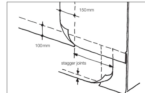
6 Lap membrane correctly. At corner situations, return membrane 300mm round external corners and fix. Membrane can be secured temporarily with tape but must be mechanically secured immediately afterwards.
