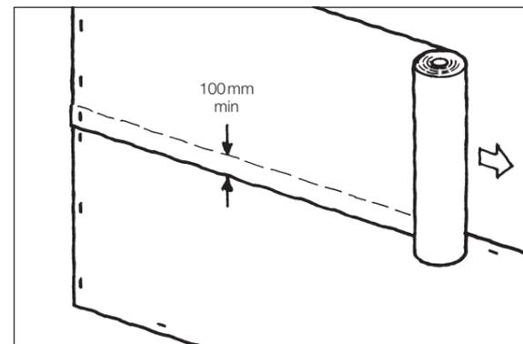
4 Fix second layer and repeat up to roof abutment. Ensure 100mm minimum horizontal laps and 150mm minimum vertical laps and seal with Protect FR tape.
