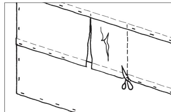
1 Replace damaged and torn membrane with a patch of membrane.
