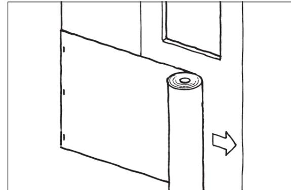
1 Unroll across substrate horizontally with the 'black' coated surface of the membrane facing outwards.
