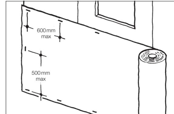
2 Secure membrane with suitable mechanical fixings at maximum 500mm vertical centres and maximum 600mm horizontal centres.
