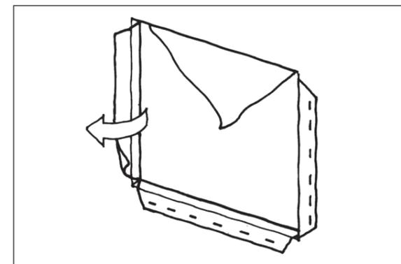
5 Dress into door and window recesses and fix with suitable mechanical fixings at 200mm centres.
