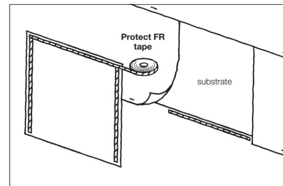
2 Patch should be lapped accordingly and sealed with Protect FR tape. It is recommended to pre-apply tape to the patch.
