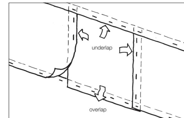
3 Once the patch is in place, tape seals should be securely pressed down and mechanical fixings applied.
