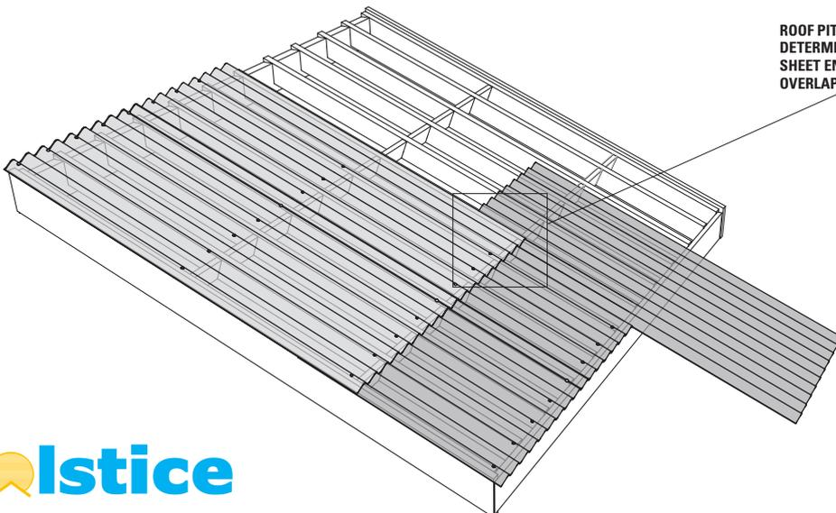
ROOF PITCH DETERMINES SHEET END OVERLAP
