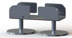
PED50—Designed to work with the 50,70, 100 and 120mm joists. The PED50 has a minimum height to the underside of the joist of 8mm, with an adjustment range of 35mm
