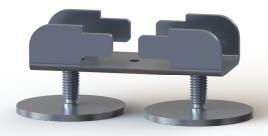
PED20XR—Designed to work with the 20mm joist, but with an extended working range. The PED20XR has a minimum height to the underside of the joist of 18mm, with an adjustment range of 22mm
