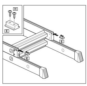
7. Loosely insert 12mm screws (H) into both stops (E) and slide into the top ladder section.
