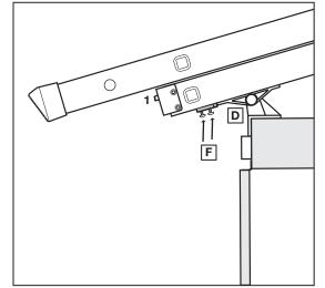
14. Release the locking catch on the top ladder section (1) and slide the bottom section up until it locks. Use the pole to fully stow the ladder. The ladder should not rest horizontally. With the ladder fully stowed, slide the retainers (F) up to the glide/pivot assembly (D) and clip onto the glide.
