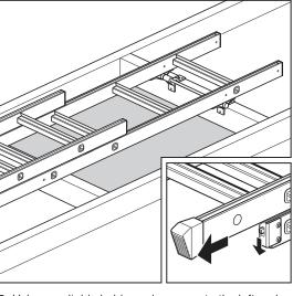
10. Using a suitable ladder, gain access to the loft and position the loft ladder centrally across the loft opening with the pivot assembly resting squarely on the trapdoor surround. To help with access, release the locking catch on the end of the top ladder section and slide the bottom section down the ladder.
