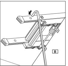
15. To lower ladder. Insert the pole (B) into the round hole on the bottom ladder section and carefully pull down until top section rests on top stops
