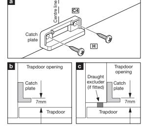
4. Attach catch plate. Find and mark the centre line onto the opening end of the trapdoor surround. Allow a 7mm gap between the top of the catch plate and the trapdoor (b or c). Attach the catch plate (C4) to the trapdoor surround using 2 x 12mm screws (a).
