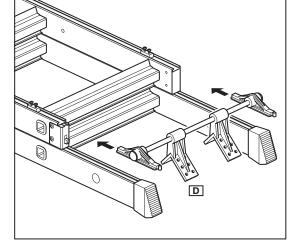
8. Slide the glide/pivot assembly (D) into the ladder, ensure it is fitted the correct way around as shown.
