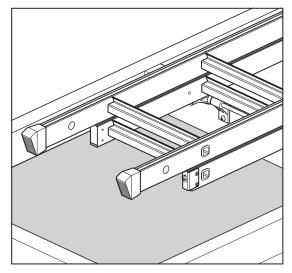
12. Close the ladder, engage the locking catch and slide the ladder into the loft so that the top section is resting horizontally on the loft floor.
