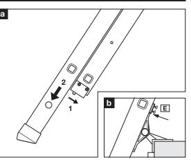
16. When ladder comes to a stop, release catch on top section (1) and lower bottom section (2) until it locks into place (a). IMPORTANT: Ensure top stops (E) are tight against glides (b) and feet sit evenly on the floor.
