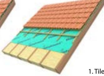
Warm Roof - OSB Sarking - Tile (Alternate Detail)
