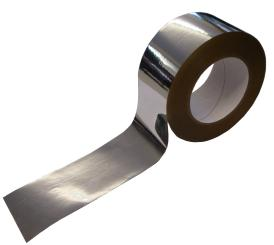
**Novia<sup>®</sup> Cold Weather Metallised BOPP tape** should be used in all AVCL and DPM applications as an edge and lap sealing tape in conjunction with the **Novia<sup>®</sup> Double Sided Butyl** sealing tape. For the best results for airtightness and prevention of interstitial condensation, Novia advises the use of both lap and butyl tapes on all AVCL and DPM installations.
