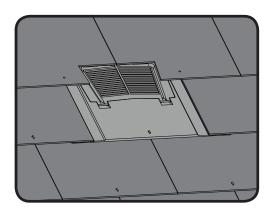
**12.** When laying the course above, some trimming of the slates directly above the vent is required to ensure they do not obstruct the grille opening.
