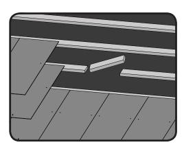
3. The installation of the vent requires at least one batten to be cut. Using the trimmed slates as a guide, mark out a 250mm wide section of the batten below and cut it out, taking care not to damage the underlay.
