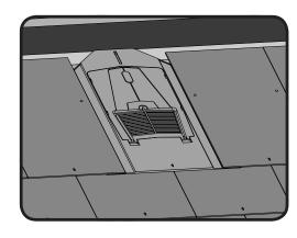
11. Fit the adjacent slates, lapping them over the edge skirt and up to the required width for the slates. For 250mm wide slates, lay to the outer guide edge, narrower slates can be overlapped up to the inner guide edge.
