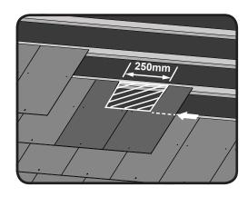
2. On the two slates, mark out an area that is 250mm wide (125mm per slate) and as far down as the top edge of the slates on the course below, as shown above.
