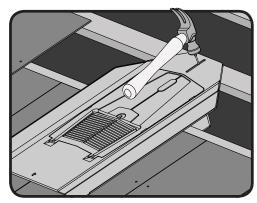
**10.** Nail the vent into position through the upper fixing slot provided. A disc rivet should be used to secure the front edge.
