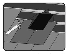
**8.** Replace the cut slates and securely fix them in position ensuring that the vent penetration is left unobstructed.
