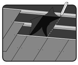
**6.** Cut the underlay along the diagonal X lines and fold back the triangular tabs to reveal the base opening.
