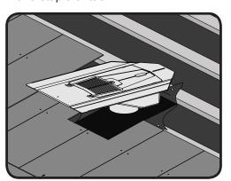
**9.** Slot the vent into position, allowing the base to pass through the underlay. Align the vent centrally with the slates below.
