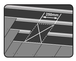
**5.** Using the trimmed batten(s) as a guide, mark a box on the underlay below, join the corners diagonally with an 'X'.
