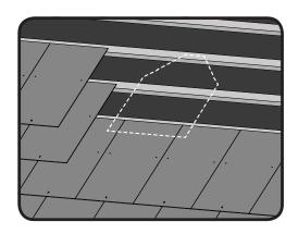
1. Prepare the roof in the conventional manner, finishing two courses below where the vent is intended to be installed. Lay the two slates on the course directly below the where the vent will be, but do not fix them in place. Vent cannot be installed over a truss or rafter.
