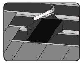
**7.** Fold the 4 tabs tight up against the adjoining battens and secure in position with a staple or tack.
