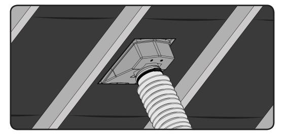
13. If you wish to use the terminal for mechanical extraction, soil stack ventilation or with other ducted ventilation systems, first install the vent as instructed and then locate the outlet within the loft space. The GILSV25-20 has an integral 4" diameter circular outlet on its base which can connect directly on to a Manthorpe GRPA Flexible Pipe. To fit, simply align the GRPA, push over the outlet and secure it in place with a jubilee clip.
