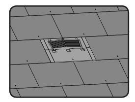
**12.** Install the slates above the vent as normal, when using larger 600 x 300mm formats there is no requirement to trim the slates above.
