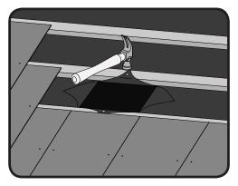
**7.** Fold the upper and lower tabs tight up against the battens and secure in position with a staple or tack.
