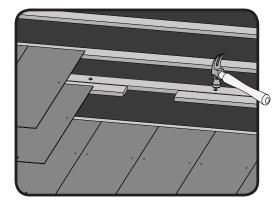
**3.** Smaller 500 x 250mm slate sizes require the batten to be cut. Using the trimmed slates as a guide, mark out the section of batten that needs to be removed and cut it out.
