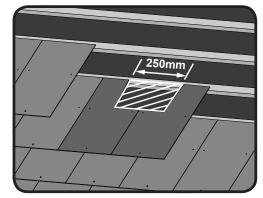
**1.** Prepare the roof in the conventional manner, finishing two courses below where the vent is intended to be installed. Lay the two slates on the course directly below the where the vent will be, but do no fix them in place.
