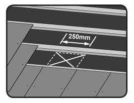
**5.** Using the trimmed slates as a guide, mark a box on the underlay below, join the corners diagonally with an 'X'.
