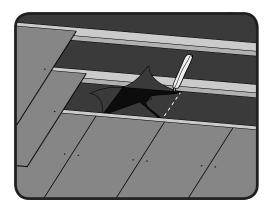
**6.** Cut the underlay along the diagonal X lines and fold back the triangular tabs to reveal the spigot opening.
