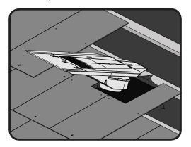
**9.** Slot the vent into position, allowing the base to pass below the batten. Align the vent centrally with the slates below.
