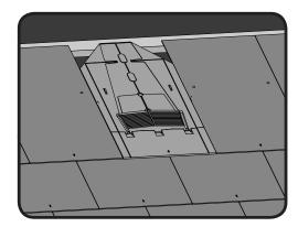
**11.** Fit the adjacent slates, lapping them over the edge skirt and up to the side of the vent (with 500 x 250mm slates trim the 2 adjacent slates down by 25mm to fit around the vent). If using disc rivets for the surrounding slates, these can be installed into the slot on the sides of the vent. Fix the adjacent slates and continue along the course in the usual manner.
