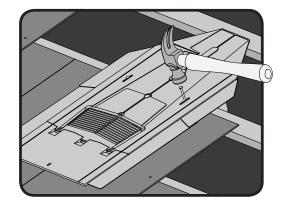
**10.** Nail the vent into position through the two fixing slots provided. A disc rivet should be used to secure the front edge.
