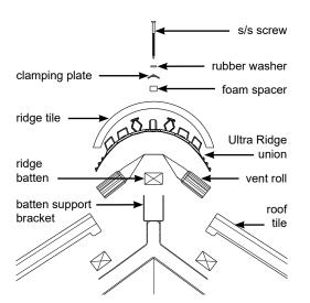
Fig B. Finished Ultra Ridge Detail
