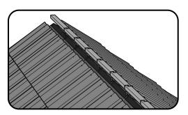
**4.** Fix the top course tiling battens and tile the roof on both sides as normal. If using a Manthorpe Dry Verge or Linear Dry Verge Systems, fix these at this stage.
