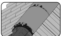
7. Lay the ridge tiles along the ridge, placing an Ultra Ridge Union between each adjacent tile.
