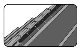
**3.** Lay a timber batten between the brackets, then bend the two up-stands over the batten and nail in place using 25mm Stainless Steel annular ringshank nails.
