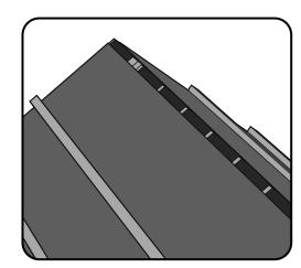
1. Lay the roofing underlay and dress it over the apex of the roof in the standard practice. Fix the battens to the roof as normal up to, but excluding, the top course of tiling battens.
