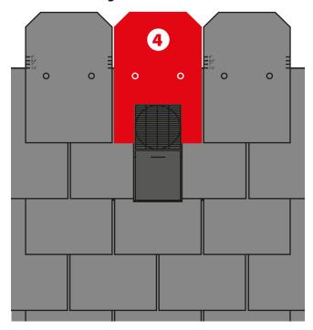
Fit cut piece 4 central over the top of the ventilator. As before, the top of the third course slates should line up with the 7.5" exposure lines on this fourth course. Secure in place using the standard nailing areas on the Tapco-Slate and then add slate courses to the side and above.
