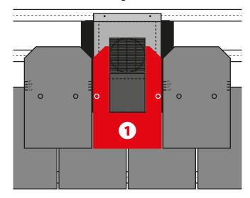
Fit cut piece 1 over the top of the ventilator. The top of the first course slates should line up with the 7" exposure lines on this second course. The non-nailable area guide should be used to locate the new nailing areas needed to secure cut piece 1, the standard nailing markers **should not be used** (nailing here would damage the ventilator).
