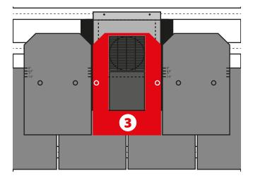
Fit cut piece 3 over the top of the ventilator. The top of the first course slates should line up with the 6" exposure lines on this second course. The non-nailable area guide should then be used to locate the new nailing areas needed to secure cut piece 3 as the standard nailing markers **should not be used** (nailing here would damage the ventilator).
