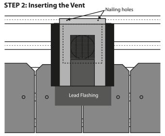
Fit the ventilator into the gap that was cut into the battens, push the unit up to the top batten and nail in place using the nailing holes provided.
