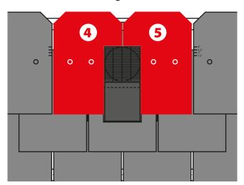
Fit cut pieces 4 and 5 centralised over the top of the ventilator. Again, the top of the second course slates should line up with the 6.5" exposure lines on this third course. The non-nailable area guide should then be used to locate the new nailing areas needed to secure cut pieces 4 and 5 on just the inside edges where the slate meets the ventilator raised centre. The standard nailing guides can be used on the outside edges which are well outside the non-nailing area.
