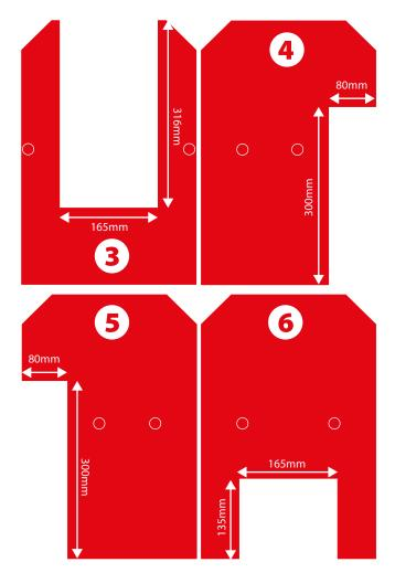
Please note that both of the TapcoSlate nailing guides on cut piece No. 3, to the right of No. 4, and to the left of No. 5 should not be used. Instead these should be nailed according to the **non-nailable area** discussed on page 1.
