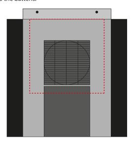
The non-nailable area is highlighted in red in the diagram above. Cut a template to the dimensions below:
