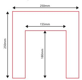
Place this template over the top of the ventilator each time you add a course of TapcoSlates and **do not** nail inside the template area.
