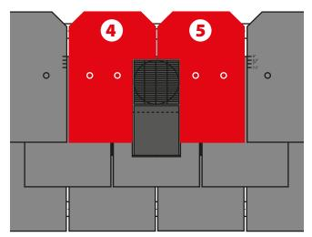
Fit cut pieces 4 and 5 centralised over the top of the ventilator. Again, the top of the second course slates should line up with the 6" exposure lines on this third course. The non-nailable area guide should then be used to locate the new nailing areas needed to secure cut pieces 4 and 5 on just the inside edges where the slate meets the ventilator raised centre. The standard nailing guides can be used on the outside edges which are well outside the non-nailing area.
