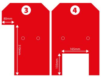
Please note that both of the TapcoSlate nailing guides on cut piece No. 1, to the right of No. 2, and to the left of No. 3 should not be used. Instead these should be nailed according to the **non-nailable area** discussed on page 1.
