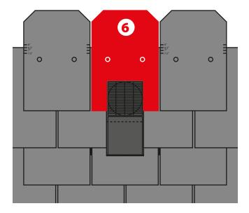
Fit cut piece 6 central over the top of the ventilator. As before, the top of the third course slates should line up with the 6.5" exposure lines on this fourth course. Secure in place using the standard nailing areas on the Tapco-Slate and then add slate courses to the side and above.
