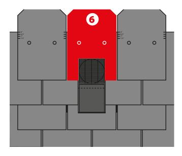
Fit cut piece 6 central over the top of the ventilator. As before, the top of the third course slates should line up with the 6" exposure lines on this fourth course. Secure in place using the standard nailing areas on the TapcoSlate and then add slate courses to the side and above.
