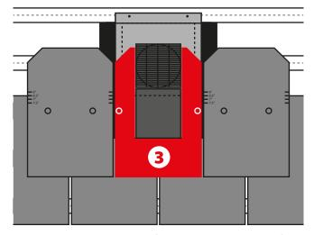
Fit cut piece 3 over the top of the ventilator. The top of the first course slates should line up with the 6.5" exposure lines on this second course. The non-nailable area guide should be used to locate the new nailing areas needed to secure cut piece 3, the standard nailing markers **should not be used** (nailing here would damage the ventilator).
