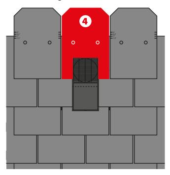
Fit cut piece 4 central over the top of the ventilator. As before, the top of the third course slates should line up with the 7" exposure lines on this fourth course. Secure in place using the standard nailing areas on the TapcoSlate and then add slate courses to the side and above.
