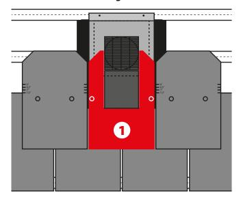
Fit cut piece 1 over the top of the ventilator. The top of the first course slates should line up with the 7.5" exposure lines on this second course. The non-nailable area guide should be used to locate the new nailing areas needed to secure cut piece 1, the standard nailing markers **should not be used** (nailing here would damage the ventilator).
