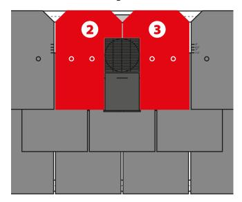
Fit cut pieces 2 and 3 centralised over the top of the ventilator. Again, the top of the second course slates should line up with the 7.5" exposure lines on this third course. The non-nailable area guide should then be used to locate the new nailing areas needed to secure cut pieces 2 and 3 on just the inside edges where the slate meets the ventilator raised centre. The standard nailing guides can be used on the outside edges which are well outside the non-nailing area.
