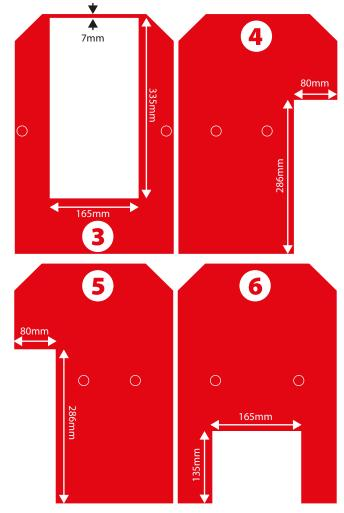
Please note that both of the TapcoSlate nailing guides on cut piece No. 3, to the right of No. 4, and to the left of No. 5 should not be used. Instead these should be nailed according to the **non-nailable area** discussed previously.
