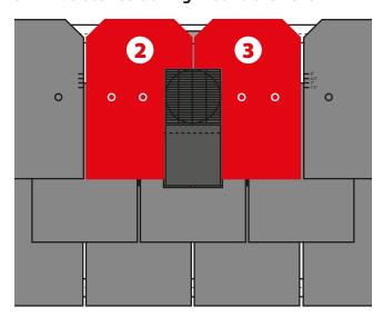
Fit cut pieces 2 and 3 centralised over the top of the ventilator. Again, the top of the second course slates should line up with the 7" exposure lines on this third course. The non-nailable area guide should then be used to locate the new nailing areas needed to secure cut pieces 2 and 3 on just the inside edges where the slate meets the ventilator raised centre. The standard nailing guides can be used on the outside edges which are well outside the non-nailing area.
