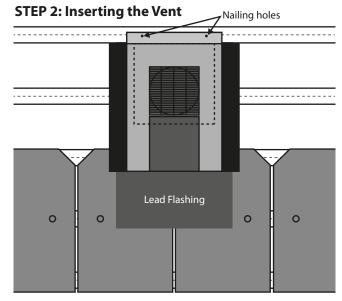
Fit the ventilator into the gap that was cut into the battens, push the unit up to the top batten and nail in place using the nailing holes provided.
