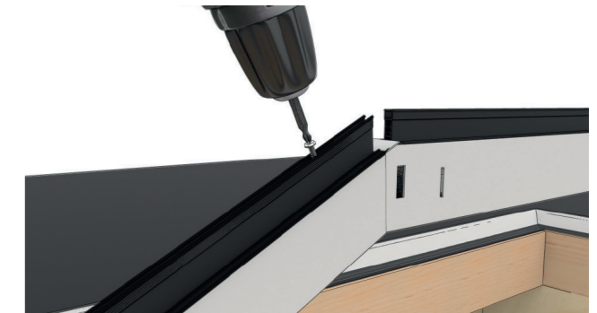
2 Secure the bell rafter using the pre-fitted retention screw.
