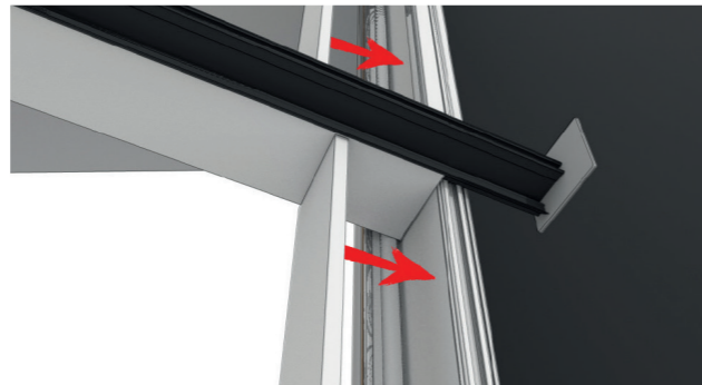
14 Use internal foamboards to space out rafter positions before fixing rafters to the ringbeam.
