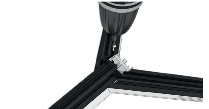
10 Tighten pre-fixed screw at the top of the hip rafter to hold bracket.
