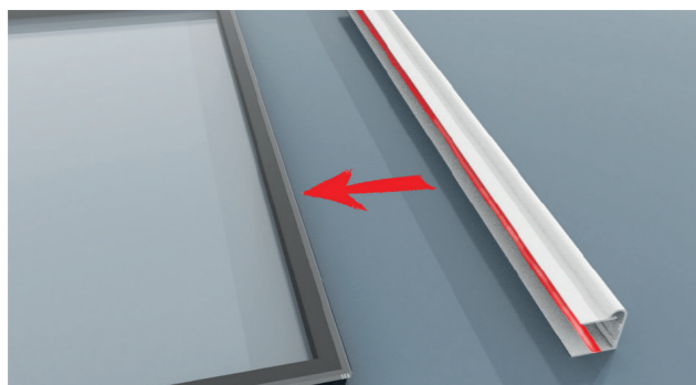
17 Apply a bead of sealant to glazing end closer and fit centrally to glass units. Note: Always use the correct polymer sealant for self cleaning glass. Illustration shows underside of glass, please note, when fitting drip faces down.
