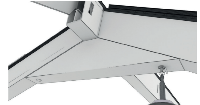
8 Secure in pre-drilled holes with supplied 5 x 70mm screws and fit cap covers.
