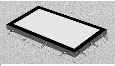
4) Secure fixing screws with horse shoe packers and finishing caps continuously all the way around securing the aluminium frame in place.
