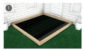
Prepare a level, weed-free area for the deck. To create a framework, cut the C24 47mm x 100mm (or 47mm x 150mm) green treated timber to the required length, then join using exterior wood screws. Check the frame is square by measuring diagonally from corner to corner. Use a weed mat to ensure weeds do not grow through from the bottom of your deck frame if needed.
