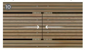
Once the boards are secure at both ends, drill a 65mm speedekz decking screw at regular intervals along all boards. If your decking boards need to butt up to another timber decking board on the length, simply butt them together with a small gap ontop of a supporting joist. Butt ends should always have supporting joists underneath to ensure the boards are adequately supported. Make sure all boards are fully stable and in place.
