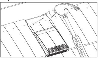
Position the ventilator with the spigot through the underlay cut and nail the ventilator to the batten through the holes in the top flange.
