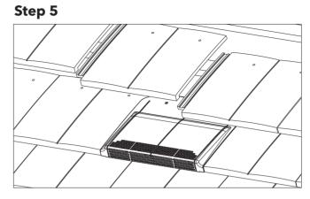
With the ventilator in position, tiling can be completed, leaving a discreet flush fitting installation.
