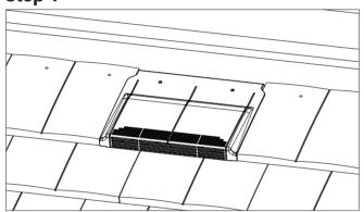
Locate the position of the ventilator in the roof, ensuring that the location is clear of the rafters below.
