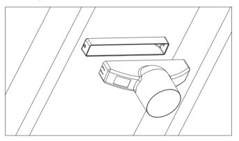
The ventilator must be accessed from the underside. Fit the Pipe Adaptor (code: HD DPCA) over the spigot on the underside of the ventilator ensuring the adaptor clips onto the spigot securely
