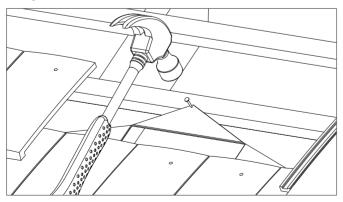
The top and side underlay triangular shapes should be folded outward and underneath the ventilator. The top triangle should be pulled tightly and tacked to the batten above.
