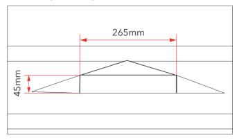
It is important that the cut forms a snug fit to the ventilator to deflect and prevent water and debris penetration through the underlay.
