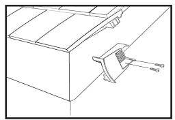
3. The verge starter unit (code: HD IPTDV/ST) should be fixed securely at the eaves through the slots using the 2 x 25mm flange head screws provided into the barge board or
