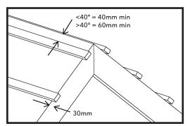
1. The tile battens should be fixed as required with a 35mm overhang beyond the face of the masonry or barge board creating a gap of 5mm or so between the verge unit and the wall or barge board. The distance between the apex and the top batten should not exceed 80mm. The underlay should be trimmed to extend 5mm beyond the ends of the battens.
