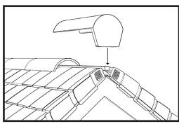
8. Alternatively, a block end ridge tile may be used to complete the installation, fitted in accordance with the tile manufacturer's recommendations. For roof pitches above 50° a block end ridge tile should be used.
