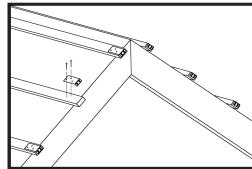
2. It is recommended that batten end clips (code: HD IDV/BC) should be used at the batten ends to provide long term secure fixing and wind load resistance to comply with BS 8612. One clip should be nailed twice to the top of each batten with the short flange in contact with the batten end.
