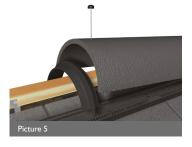
7) Continue fixing nailhole ridge tiles, top fillers and ridge seals along the ridge. If cutting is necessary to maintain the aesthetics of the ridge line, the block end ridge must not be cut. Ridge tiles must not be cut to less than half of their original length. All ridge tiles must be twice fixed with drive screws supplied (re-drill nailholes if necessary). At the verge, trim the last top fillers and fix the block end ridge tile as described in step 6 to finish the ridge line (Picture 6).
