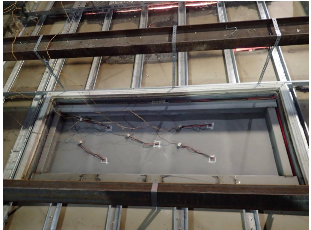
The unexposed face of the test assembly after a test duration of 120 minutes, showing Hatch A
