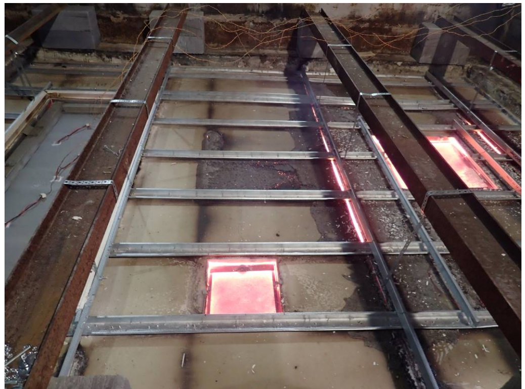
The unexposed face of the test assembly after a test duration of 120 minutes, showing Hatch B
