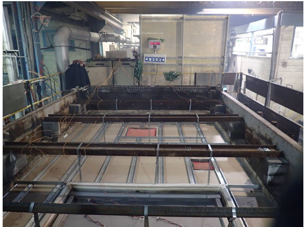
The unexposed face of the test assembly after a test duration of 40 minutes
