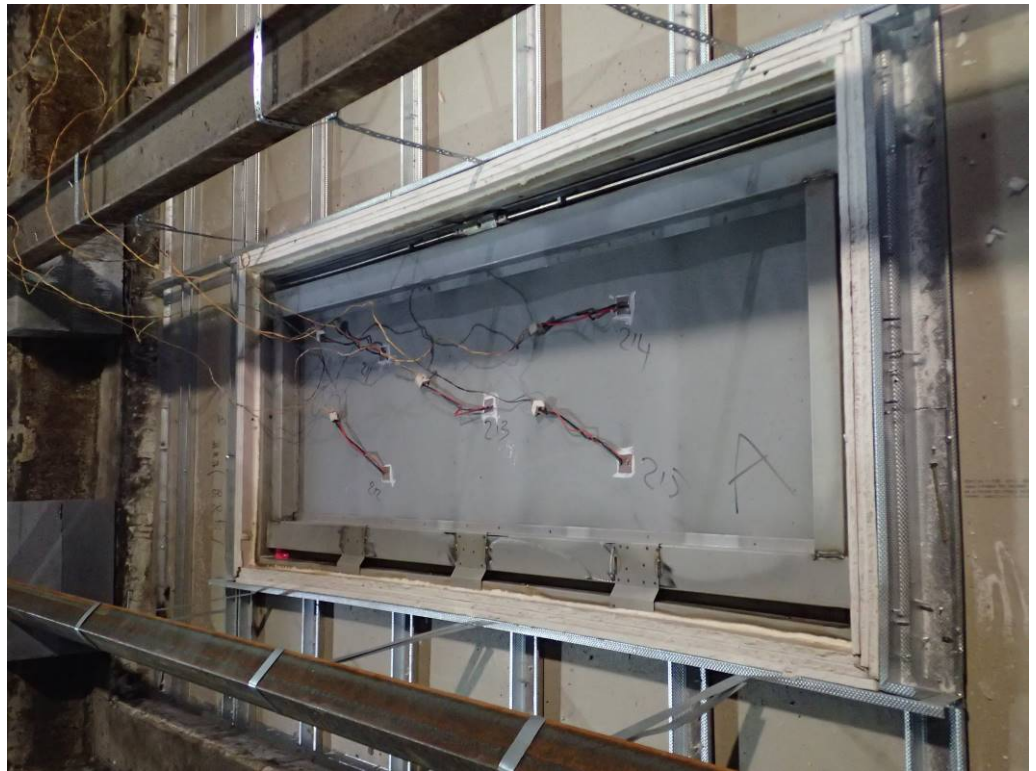
The unexposed face of the test assembly after a test duration of 60 minutes, showing Hatch A
