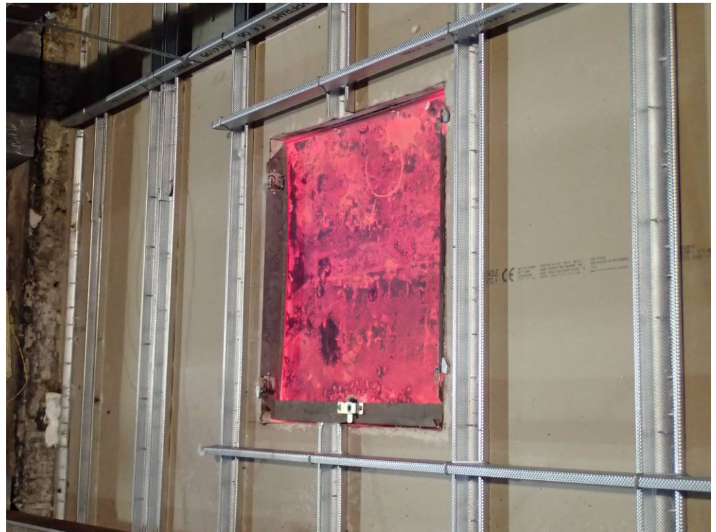
The unexposed face of the test assembly after a test duration of 60 minutes, showing Hatch C
