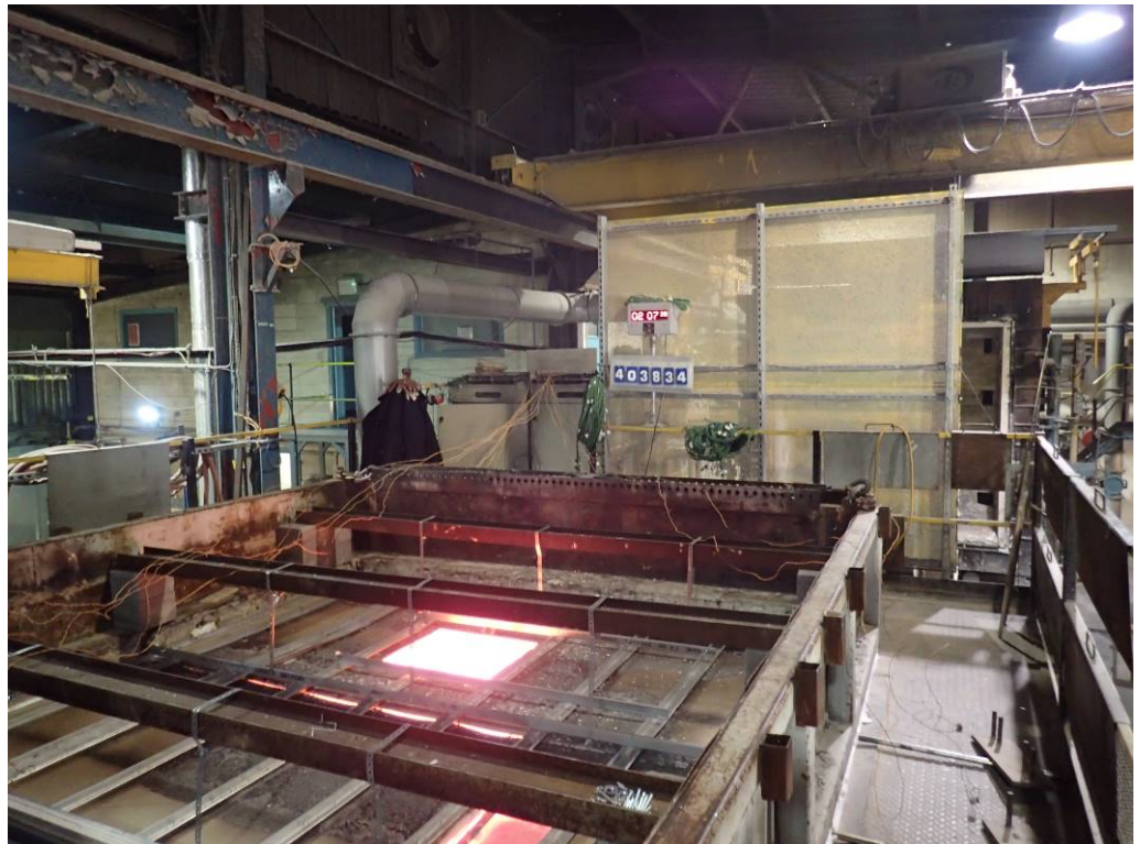
The unexposed face of the test assembly after a test duration of 127 minutes
