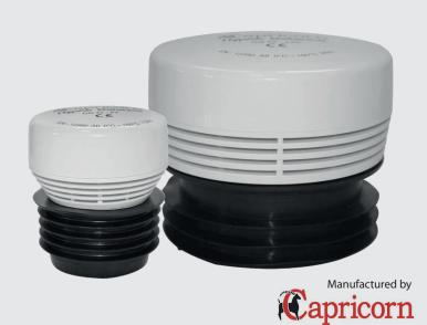
Air Admittance Valves (AAV's) allow air to freely enter the sanitary pipe work system and prevents the escape of foul gases into the building. They are suitable for 32-110mm waste and soil pipes.
