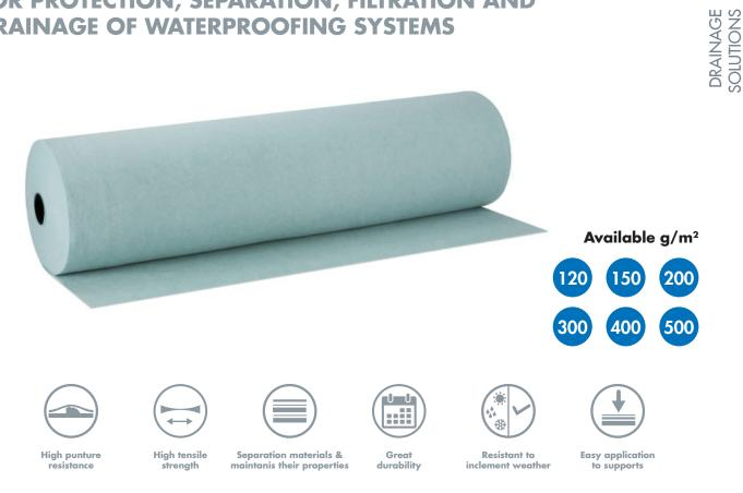
DANOFET<sup>®</sup> PY is a non-woven geotextile formed by polyester threads, interwoven by needling, without the need or application of chemical binders. It has excellent mechanical and hydraulic behavior.
