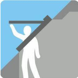
A top-hung roof window is ideal if you have to, or wish to, place your window at high level, for instance in connection with a high knee wall.
