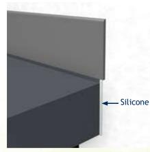
Optional: seal sides with a highquality low modulus silicone i.e., Dow Corning or Adshead Ratcliffe colour matched to the same colour as the canopy, alternatively use a translucent colour.
