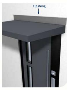
**8.** Finally, dress the top of canopy with lead or required flashing.
