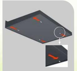
**4** Assemble top section and soffit section with 4 self-tapping screws.
