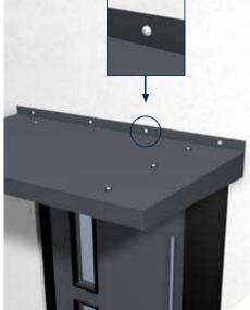
7b. Fix though the upstand into the wall.
