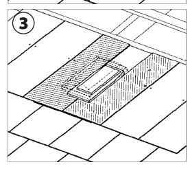
1. Lay slates to the required position of the ventilator. Cut the slate directly below the ventilator so that it does not protrude past the slate batten. Cut a 280mm wide gap in the batten at the head of the slate as shown.
