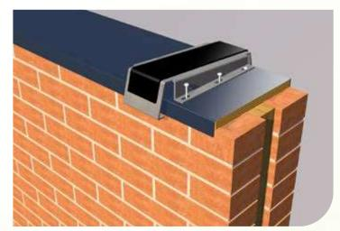
3. Position bracket with EPDM seal centrally over the wall. Maintain a minimum 10mm gap from the bracket inside return edge to the external wall surface finish (see Point 4 and also refer to Point 7). Brackets should be spaced at the correct centres according to the recommended number of brackets (please refer to Skyline technical data for information).
