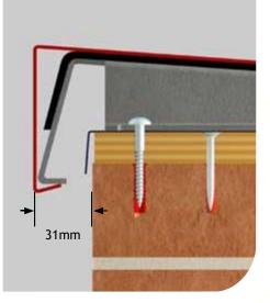
7. Ensure 31mm dimension is maintained from external wall surface finish to external face of coping. On deeper edged coping that exceeds the normal 85mm leg, it may be necessary to use a small self-tapper on the coping return to secure it fully.
