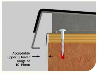
4. Secure coping bracket with high quality fixing (minimum 50mm) appropriate for the substrate. The bracket has pre-drilled fixing holes which are provided as guidance only. Use the outermost fixing points to ensure maximum anchor point of the bracket to the wall. If fixings penetrate the masonry below, then ensure that the fixing is sufficiently back from the face to avoid damaging the masonry.
