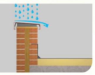
2. Skyline Sloping Coping is manufactured with an integral 20mm fall. Always install with the fall sloping towards the roof area. This ensures that rainwater run-off will be directed back onto the roof area.
