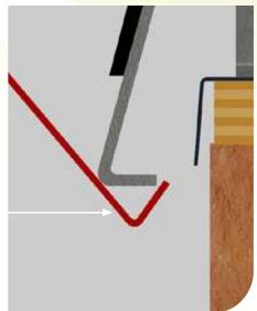
6. The coping simply pivots over the coping brackets and clips into position. First locate the front edge, and pivot over the bracket whilst slowly pressing the coping section into place to compress the EPDM seal on the brackets. Expect some resistance and apply consistent pressure and continue to press until it clips over the other edge of the bracket. The same method applies to corners, T-junctions and stop ends.
