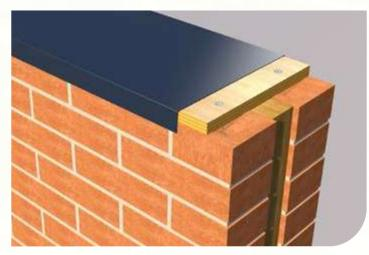
1. Ensure minimum 18mm marine ply and weatherproof membrane is fitted to the structure before commencing with the installation (all supplied by others).
