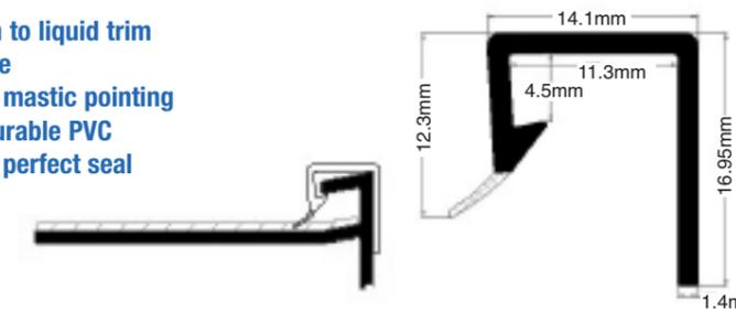
Glasstrim, V-Trim GRP, Driptrim and Rofycom are pultruded glass reinforced polyester roof edge trims, designed to provide a strong, weather-proof, decorative roof edge finish and create a waterproof bond. They can be used with felt roofing, asphalt and liquid roofing systems.
