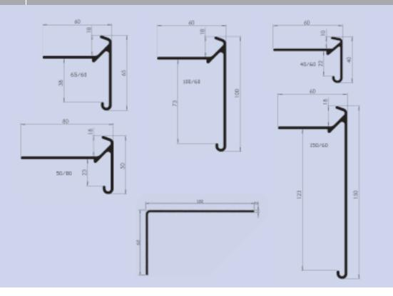
Glasstrim, V-Trim GRP, Driptrim and Rofycom are pultruded glass reinforced polyester roof edge trims, designed to provide a strong, weather-proof, decorative roof edge finish and create a waterproof bond. They can be used with felt roofing, asphalt and liquid roofing systems.
