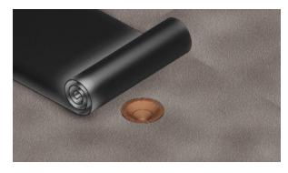
**Step 2**Lay new vapour barrier & bond into existing rainwater outlet.
