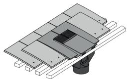
The vent outlet is designed to penetrate through the roofing underlay between the tile courses, meaning there is no need to cut or trim the battens, even when laid at the lowest batten gauge of 88mm (when using 38mm roofing battens).
