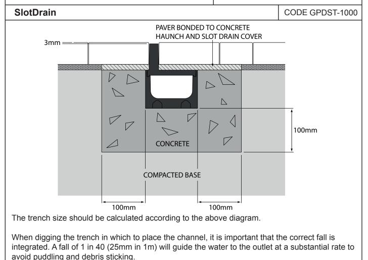
The concrete used should be no less than a C25 strength mix, which when fully cured will withstand 25 N/mm<sup>2</sup> of compressive force.
