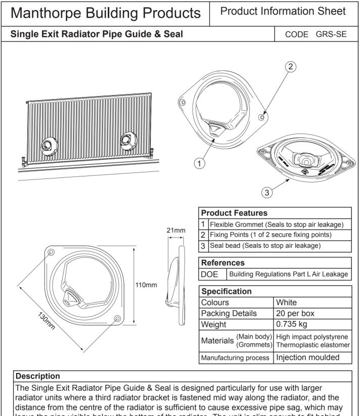
leave the pipe visible below the bottom of the radiator. The unit is slim enough to fit behind the radiator and will provide a draught seal to help achieve the new air leakage requirements of the modern building regulations. Due to its face-fix nature, the product is ideal for studded wall details.
