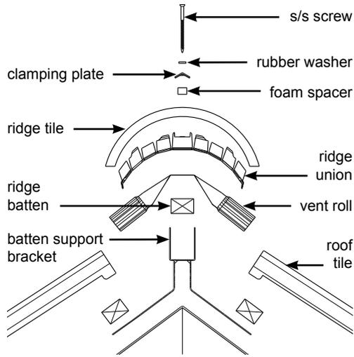
**Fig B. Finished Dry Ridge Detail**
