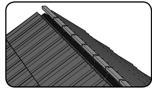
**4.** Fix the top course tiling battens and tile the roof on both sides as normal. If using a Manthorpe Dry Verge or Linear Dry Verge Systems, fix these at this stage.
