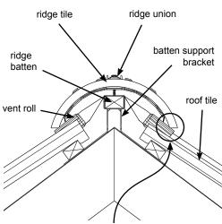
NOTE: Vent roll should extend at least 5mm beyond the contact point of the ridge tile.
