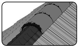
**7.** Lay the ridge tiles along the ridge, placing a Ridge Union between each adjacent tile.
