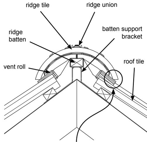
**NOTE:** Vent roll should extend at least 5mm beyond the contact point of the ridge tile.
