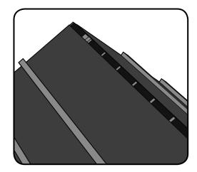
1. Lay the roofing underlay and dress it over the apex of the roof in the standard practice. Fix the battens to the roof as normal up to, but excluding, the top course of tiling battens.
