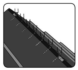
2. Adjust the height of the brackets by bending the bracket at the appropriate height (1-4) as indicated in tables 1-3 overleaf.
