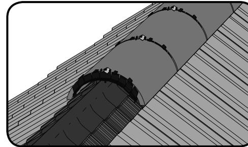
**7.** Lay the ridge tiles along the ridge, placing a Ridge Union between each adjacent tile.
