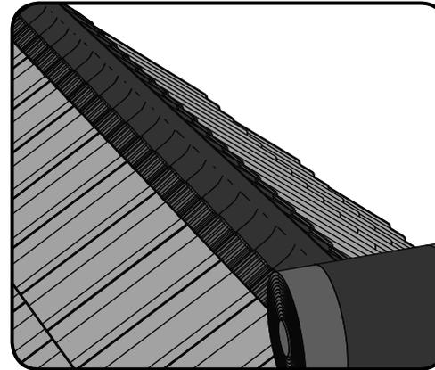
**5.** Roll out the Vent Roll along the entirety of the ridge, tacking the roll at 1m intervals to the ridge batten using staples or felt nails.
