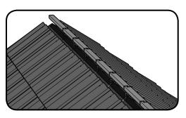
**4.** Fix the top course tiling battens and tile the roof on both sides as normal. If using a Manthorpe Dry Verge or Linear Dry Verge Systems, fix these at this stage.
