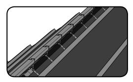
**3.** Lay a length of timber batten between the Support Brackets, then bend the two upstands over the batten and nail in place.
