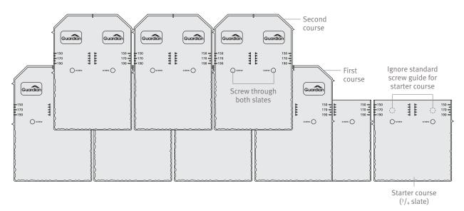
6. Fasten each Guardian Slate with two 30mm x 4mm head stainless steel screws.
