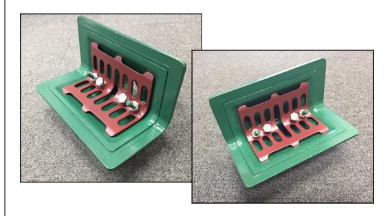
Caroflow Mini Two-Way Threaded Roof Outlet is designed for use at the intersection of horizontal and vertical surfaces, i.e. a balcony and parapet wall, and can be used to drain off vertically or horizontally. Available in either LM6 Aluminium Silicon casting alloy to BS EN 1706:2010 for most roof finishes or in leaded gunmetal to BS EN 1982:2008 for use with lead or copper-clad roofs or for connection to copper pipe work. They are female parallel threaded to BS21:1985.
